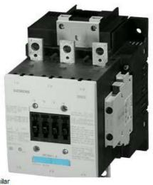
CONTACTOR, 75KW/400V/AC-3, AC(40...60HZ)/DC OPERATION UC 500...550V AUXIL. CONTACTS 2NO+2NC 3-POLE, SIZE S6 BAR CONNECTIONS CONVENTIONAL OPERATING MECHAN. SCREW TERMINAL
