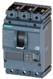
CIRCUIT BREAKER 3VA2 IEC FRAME 100 BREAKING CAPACITY CLASS C ICU=110KA @ 415 V 3POLE, LINE PROTECTION ETU850, LSI, IN=25A OVERLOAD PROTECTION IR=10A ...25A SHORT CIRCUIT PROTECTION ISD=0,6..10X IN, II=1,5..12X IN NEUTRAL PROTECTION OPTIONAL WITH EXT. CT,UPTO 160% BUSBAR CONNECTION
