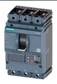
CIRCUIT BREAKER 3VA2 IEC FRAME 100 BREAKING CAPACITY CLASS H ICU=85KA @ 415 V 3POLE, LINE PROTECTION ETU860, LSIG, IN=40A OVERLOAD PROTECTION IR=16A ...40A SHORT CIRCUIT PROTECTION ISD=0,6..10X IN, II=1,5..12X IN NEUTRAL PROTECTION OPTIONAL WITH EXT. CT,UPTO 160% GROUNDFAULT, SWITCHABLE IG=0,2... 1 X IN, TG=0,050,8MS BUSBAR CONNECTION
