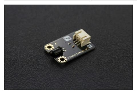
This sensor uses Gravity interface, and works from 3.3V-5V which is able to be compatible with various platforms such as Arduino, Raspberry Pi, Intel Galileo, Curie and Joule.
