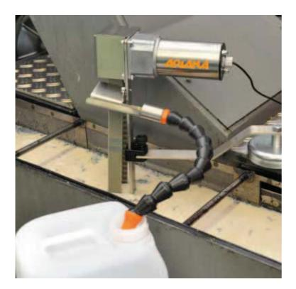
The Bandskimmer is fixed above the liquid tank by means of a magnetic disk, preferably on the opposite side of the liquid inlet. The base plate of the drive unit must be attached about 300 mm above the highest liquid level. The hose is connected to the outlet neck and guided to the sediment basin.
