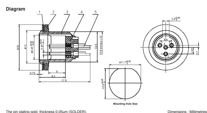
The pin plating gold, thickness 0.05µm (SOLDER).
