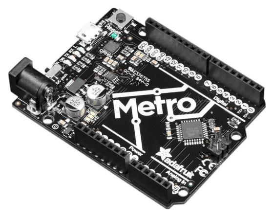
The ATmega328 processor has plenty of GPIO, Analog inputs, hardware UART SPI and I2C, timers and PWM galore – just enough for most simple projects.
