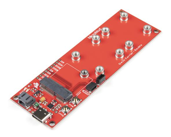
The MicroMod Qwiic Carrier Board can be used to rapidly prototype with other Qwiic devices. The MicroMod M.2 socket provides users the freedom to experiment with any processor board in the MicroMod ecosystem. This board also features two Qwiic connectors and eight 4-40 screw inserts to connect and mount Qwiic devices.
