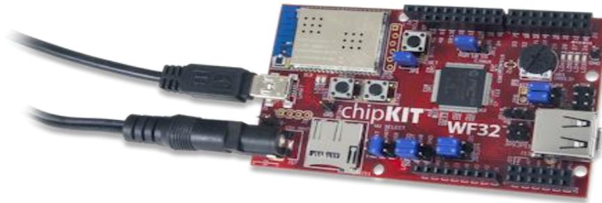
*With just the chipKIT WF32, you'll have a WiFi module, a Micro SD card slot, USB 2.0, a potentiometer, and 4 LEDs all at your disposal.*
