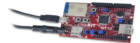
With just the chipKIT WF32, you'll have a WiFi module, a Micro SD card slot, USB 2.0, a potentiometer, and 4 LEDs all at your disposal.
