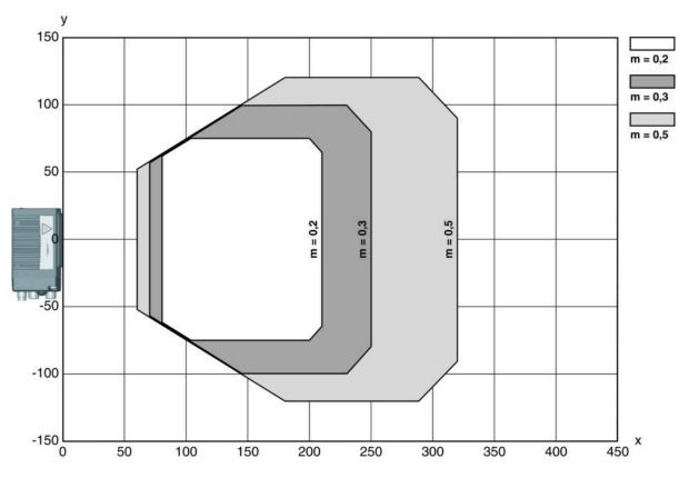
Reading field distance [mm] Reading field width [mm] x y
