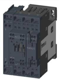
2NO+2NC CONTACTOR, AC3: 11KW DC 220V 50HZ, 240V 60HZ 4-POLE, 2NO+2NC, SZ: S0, SPRING-LOADED TERMINAL 1NO+1NC INTEGR.
