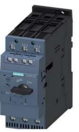
CIRCUIT BREAKER, SIZE S2, FOR MOTOR PROTECTION, CLASS 10, A-RELEASE 22...32A, N-RELEASE 416A, SCREW TERMINAL, INCREASED SWITCHING CAPACITY W. TRANSV. AUX. SWITCH 1NO+1NC
