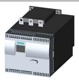
SIRIUS SOFT STARTER, VALUES WITH 690 V, 40 DEG., STANDARD: 134A, 132KW, INSIDE-DELTA CIRCUIT 3: ONLY UP TO 600V, 400-690 V AC, 230 V AC, SCREW TERMINALS
