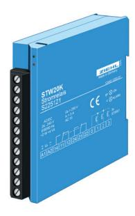
The current relay STW20K monitors the current in up to 3 lines with current transformers STWA1 (AND circuit). If there is a current in all 3 monitored lines, the relay (2 change-overcontacts) picks up. If there is no current in at least one of the lines, the relay releases. The relay works in closed circuit current. When voltage is applied to the STW, the relay signals an alarm until the it has picked up.
