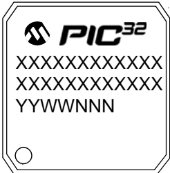
100-Lead TQFP (14x14x1 mm)
