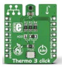
**Thermo 3 click** carries <u>TMP102</u>, a digital temperature sensor IC with a tiny footprint of only 1.6mm x 1.6mm. The click is designed to run on a 3.3V power supply only. It communicates with the target MCU through mikroBUS<sup>™</sup> I2 C pins (SCL, SDA), and an additional Alert pint (INT on the default mikroBUS<sup>™</sup> configuration).
