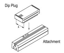
: For Crimping DIP-PLUG Distance A - 0.1" 0.3" & 0.6" (Within 40 Pins)
