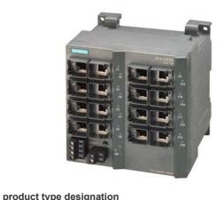
SCALANCE X216, managed IE switch, 16x 10/100 Mbit/s RJ45 ports, LED diagnostics, error-signaling contact with set pushbutton, redundant power supply, PROFINET IO device, network management, Redundancy Manager integrated, incl. electron. manual on CD-ROM, C-PLUG optional.
