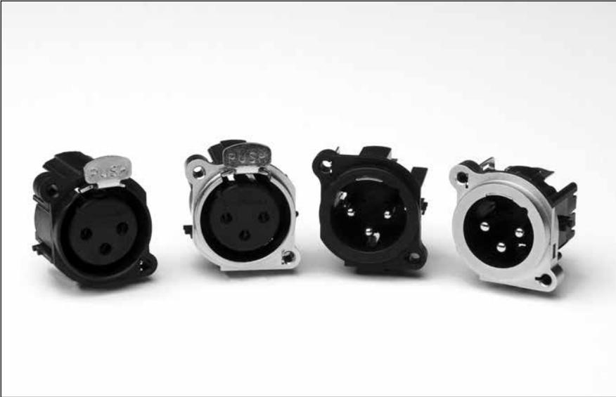
The AC series, A and B type XLR chassis receptacles have been designed and manufactured with the Original Equipment Manufacturers' (OEM) needs in mind. The compact shell design allows a significant space saving over the traditional 'D' type shell. Gold plated contacts improve the performance, ensuring a reliable contact and the unique grounding link options offer flexibility in design.
