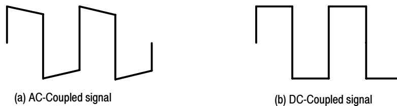
Figure 3-2: Effect of AC or DC coupling on low-frequency signals
