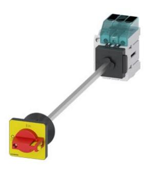
Switch disconnector 3LD3, main switch 3-polig, lu 25A operational switch at AC-23 A at 400 V 9,0 kW floor mounting Base mounting with door coupling center-hole 22,5 mm knob-operated mechanism red/yellow 48 x 48 mm with auxiliary 1NO+1NC
