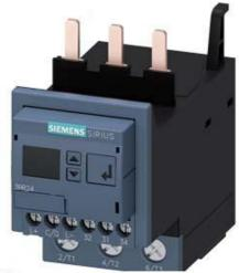
CURRENT MONITORING RELAY MOUNTABLE ON CONT. 3RT2, SZ. S2, APPARENT/ACTIVE CURR. MONIT. 8 - 80A, 20-400 HZ, 3-PH., SUPPLY 24 V DC, 1 CO CONTACT, MONITORING F. CURRENT OVER/UNDERSHOOT, CURRENT ASYMMETRY, PHASE FAILURE / WIRE BREAK, PHASE SEQUENCE, FAULT CURRENT, BLOCKING CURRENT, SWITCHING CYCLE/OP. HOURS COUNTER, WARNING/ALARM THRESHOLDS, AUTO OR MANUAL RESET ONDELAY 0-999.9 S OFF-DELAY 0-999.9 S RECLOSING DELAY 0-999.9MIN SCREW CONNECTION
