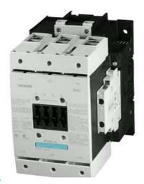
CONTACTOR, 55KW/400V/AC-3 AC(40...60HZ)/DC OPERATION UC 110...127V AUXIL. CONTACTS 2NO+2NC 3-POLE, SIZE S6 WITH BOX TERMINALS CONVENTIONAL OPERATING MECHAN. SCREW TERMINAL
