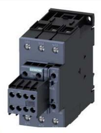
CONTACTOR,AC3:18.5KW/400V, 2NO+2NC,400VAC50HZ/400.440V60HZ 3-POLE, SIZE S2, SCREW TERMINAL
