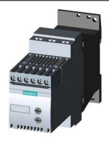
SIRIUS SOFT STARTER, SIZE S00, 12.5A, 5.5KW/400V, 40 DEGREES, 200-480V AC, 110-230V AC/DC, SCREW TERMINALS
