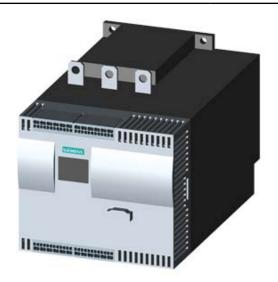
SIRIUS SOFT STARTER, VALUES WITH 400 V, 40 DEG., STANDARD: 134A, 75KW, INSIDE-DELTA CIRCUIT 3: 232A, 132KW, 200-460 V AC, 230 V AC, CAGE CLAMP TERMINALS
