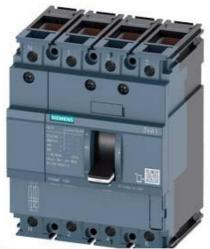
CIRCUIT BREAKER 3VA1 IEC FRAME 100 BREAKING CAPACITY CLASS S ICU=36KA @ 415 V 4-POLE, LINE PROTECTION TM210, FTFM, IN=80A OVERLOAD PROTECTION IR=80A FIXED SHORT CIRCUIT PROTECTION II=10 X IN NEUTRAL UNPROTECTED CABLE CONNECTION
