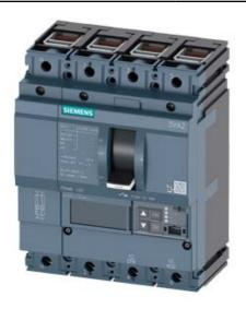
CIRCUIT BREAKER 3VA2 IEC FRAME 100 BREAKING CAPACITY CLASS H ICU=85KA @ 415 V 4POLE, LINE PROTECTION ETU860, LSIG, IN=100A OVERLOAD PROTECTION IR=40A ...100A SHORT CIRCUIT PROTECTION ISD=0,6..10X IN, II=1,5..12X IN NEUTRAL PROTECTION ADJUSTABLE (OFF, UPTO 100%) GROUNDFAULT, SWITCHABLE IG=0,2... 1 X IN, TG=0,050,8MS CABLE CONNECTION
