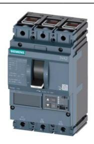
CIRCUIT BREAKER 3VA2 IEC FRAME 100 BREAKING CAPACITY CLASS M ICU=55KA @ 415 V 3POLE, LINE PROTECTION ETU560, LSIG, IN=40A OVERLOAD PROTECTION IR=16A ...40A SHORT CIRCUIT PROTECTION ISD=0,6..10X IN, II=1,5...12X IN NEUTRAL PROTECTION OPTIONAL WITH EXT. CT,UPTO 160% GROUNDFAULT, SWITCHABLE IG=0,2... 1 X IN, TG=0,050,8MS CABLE CONNECTION
