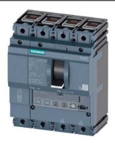
CIRCUIT BREAKER 3VA2 IEC FRAME 160 BREAKING CAPACITY CLASS C ICU=110KA @ 415 V 4POLE, LINE PROTECTION ETU350, LSI, IN=100A OVERLOAD PROTECTION IR=40A ...100A SHORT CIRCUIT PROTECTION ISD=1,5... 10 X IR, II=12 X IN NEUTRAL PROTECTION ADJUSTABLE(OFF,50%,100%) CABLE CONNECTION
