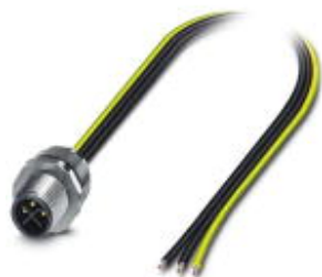
Flush-type connector, Power, 3-position, PlugLink:M12, S power, Front mounting, M16 x 1.5, Individual wires, Cable length: 0.5 m
