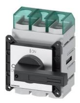
SENTRON, Molded case switch 3LD5 UL, Main switch, 3-pole, certified according to UL489 UL60947-4-1 and IEC60947-3, UL: 150A, SCCR 50kA at 480VAC, Operating power at 480VAC 3-phase: 100hp, IEC: 160A, Operating power at AC-23A at 400V: 75kW, front-mounted, rotary operating mechanism, black, 4-hole mounting of the handle, incl. terminal covers for the infeed side
