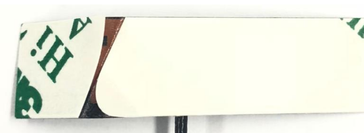
2. Bend flex slight along cut line
