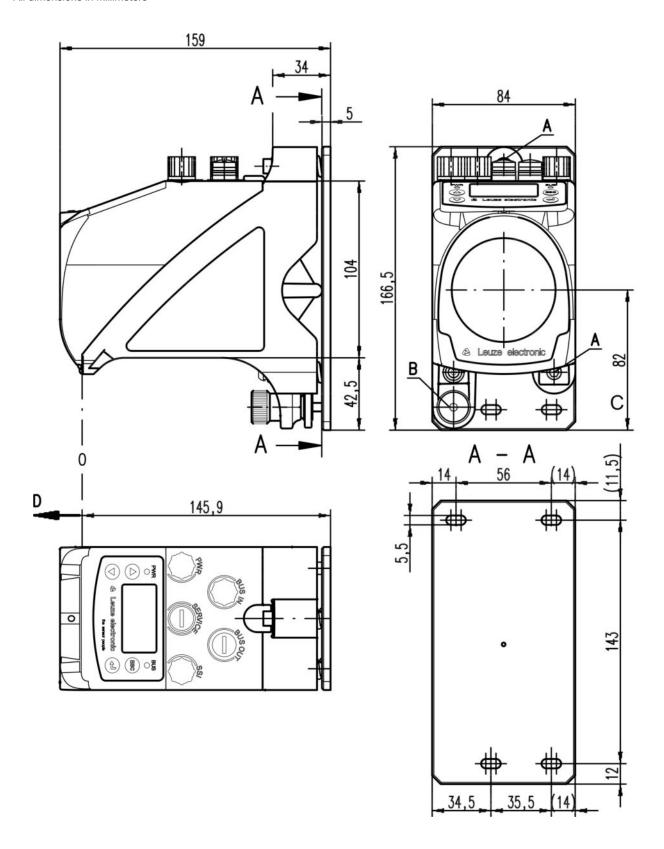
A M 5 screw for alignment
