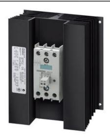
SEMI-CONDUCTOR CONTAC.3-PH.3RF2 AC51 50A 40 DEG. C 48-600V / 230V AC 3-PHASE CONTROLLED SCREW TERMINAL BLOCKING VOLTAGE 1200V
