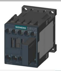
COUPLING RELAY, AC-3, 4KW/400V, 1NC, DC 24V, 0.85...1.85\*US, W. PLUGGED-ON VARISTOR 3-POLE SZ S00, SCREW TERMINAL
