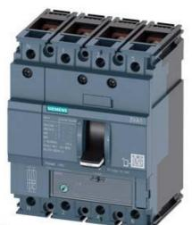
CIRCUIT BREAKER 3VA1 IEC FRAME 160 BREAKING CAPACITY CLASS S ICU=36KA @ 415 V 4-POLE, LINE PROTECTION TM220, ATFM, IN=160A OVERLOAD PROTECTION IR=112A ...160A SHORT CIRCUIT PROTECTION II=10 X IN NEUTRAL UNPROTECTED BUSBAR CONNECTION
