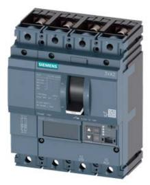
CIRCUIT BREAKER 3VA2 IEC FRAME 160 BREAKING CAPACITY CLASS C ICU=110KA @ 415 V 4POLE, LINE PROTECTION ETU550, LSI, IN=40A OVERLOAD PROTECTION IR=16A ...40A SHORT CIRCUIT PROTECTION ISD=0,6..10X IN, II=1,5..12X IN NEUTRAL PROTECTION ADJUSTABLE (OFF, UPTO 160%) BUSBAR CONNECTION
