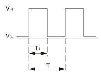
V<sub>IH</sub>=4.75 V to 5.25 V V<sub>IL</sub>=0 V to 0.4 V PWM duty cycle (%) =  $\frac{T1}{T} \times 100$  PWM frequency 25 (kHz) =  $\frac{1}{T}$  Source current (Isource) : 1 mA max. at control voltage 0 V Sink current (Isink) : 1 mA max. at control voltage 5.25 V
