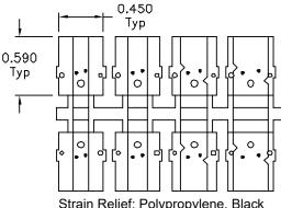
Strain Relief: Polypropylene, Black Durometer 70-Type D
