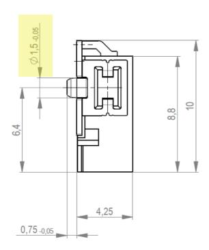
For the following article numbers we adapted the tolearance of the pig length: new 0,75mm - 0.1mm (old 0.75mm - 0.05mm)
