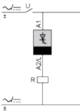
Function A : Power on Delay Relay
