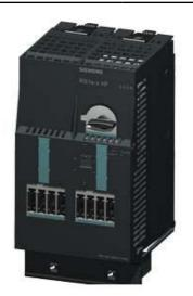
F-RS1E-X FOR ET 200S FAILSAFE REVERSING STARTER SETTING RANGE 0.3...3A MECHANICAL SWITCHING ELECTRONIC PROTECTION EXPANDABLE FOR BRAKE CONTROL MODULE 2DI MODULE 2DI MODULE SIGNAL FROM CIRCUIT-BREAKER PARAMETERIZABLE
