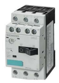
CIRCUIT-BREAKER SIZE S00, FOR MOTOR PROTECTION, CLASS 10, A-REL. 1.8...2.5A, N-REL. 33A SCREW TERMINAL, STANDARD SWITCHING CAPACITY, W. TRANSV. AUX. SWITCH 1NO+1NC
