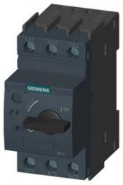
SPECIAL TYPE CIRCUIT BREAKER SIZE S00, FOR MOTOR PROTECTION, CLASS 10, A-RELEASE 9..12.5A, SHORT-CIRCUIT RELEASE 163A, SCREW TERMINAL, STANDARD SWITCHING CAPACITY AMBIENT TEMPERATURE -50 DEGREES C 500 SWITCHING CYCLES
