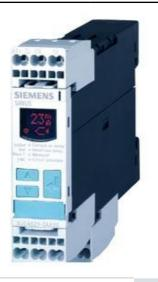
DIGITAL MONITORING RELAY CURRENT MONITORING, 22.5MM FROM 0.05 TO 10A AC/DC OVERSHOOT AND UNDERSHOOT AC/DC 24 TO 240V DC AND AC 50 TO 60 HZ STARTUP AND INTERF. PEAK DELAY 0.1 TO 20S HYSTERESIS 0.01 TO 5A 1 CHANGEOVER CONTACT W. OR W/O ERROR LOG SPRING-LOADED TYPE
