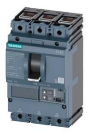
CIRCUIT BREAKER 3VA2 IEC FRAME 160 BREAKING CAPACITY CLASS H ICU=85KA @ 415 V 3POLE, LINE PROTECTION ETU860, LSIG, IN=25A OVERLOAD PROTECTION IR=10A ...25A SHORT CIRCUIT PROTECTION ISD=0,6..10X IN, II=1,5..12X IN NEUTRAL PROTECTION OPTIONAL WITH EXT. CT,UPTO 160% GROUNDFAULT, SWITCHABLE IG=0,2... 1 X IN, TG=0,050,8MS CABLE CONNECTION
