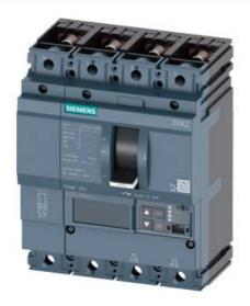
CIRCUIT BREAKER 3VA2 IEC FRAME 250 BREAKING CAPACITY CLASS H ICU=85KA @ 415 V 4POLE, LINE PROTECTION ETU850, LSI, IN=160A OVERLOAD PROTECTION IR=64A ...160A SHORT CIRCUIT PROTECTION ISD=0,6..10X IN, II=1,5..12X IN NEUTRAL PROTECTION ADJUSTABLE (OFF, UPTO 160%) BUSBAR CONNECTION
