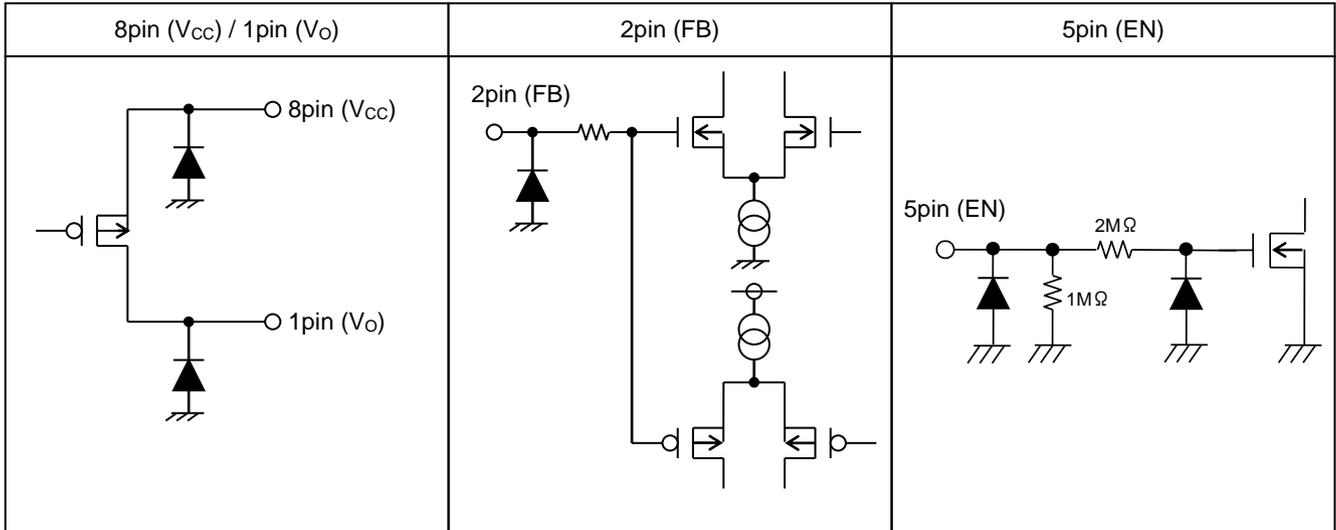
● I/O Equivalent Circuits (Output Voltage Fixed type)
